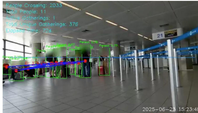
Fig. 7. Queue detection with the RoboAPP CV pipeline.
